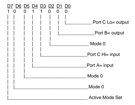
This corresponds to 98 hex. If the card address is 2D0 hex, use the BASIC OUT command to write to the control register as follows:
