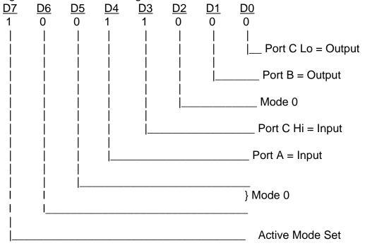
This corresponds to 98 hex. If the card base address is 2D0 hex, use the C command to write to the control register as follows:
