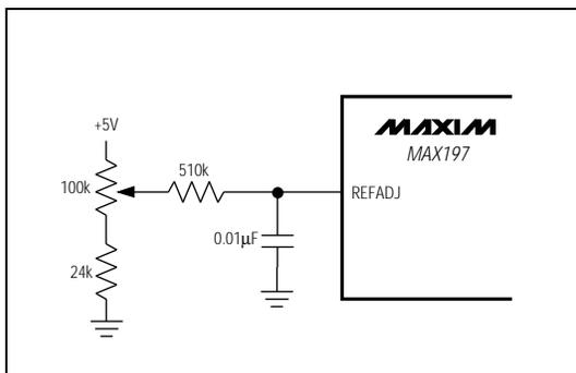
Figure 1. Reference-Adjust Circuit
