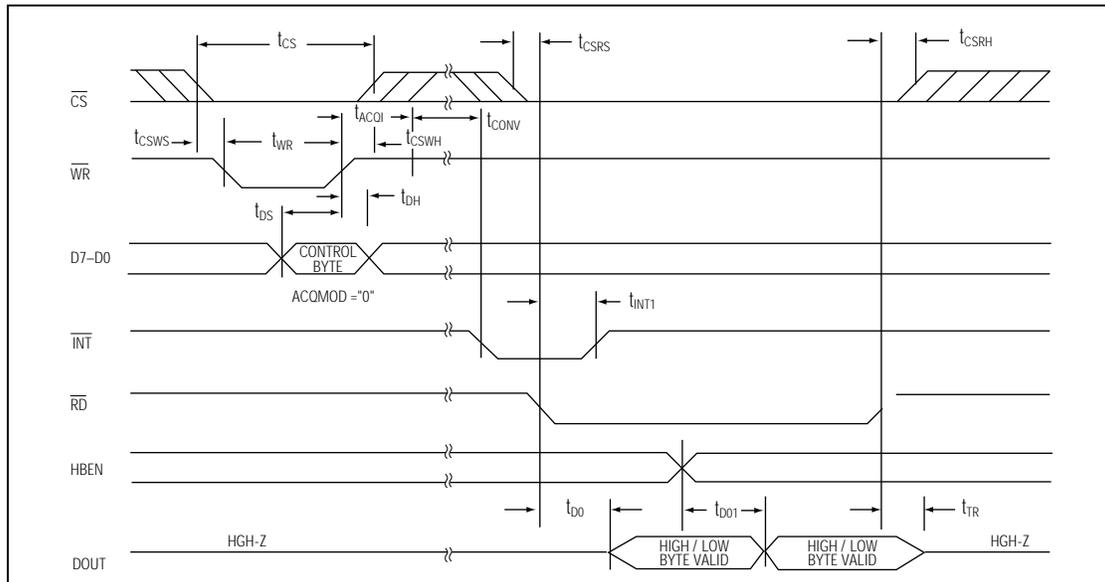
Figure 5. Conversion Timing Using Internal Acquisition Mode
