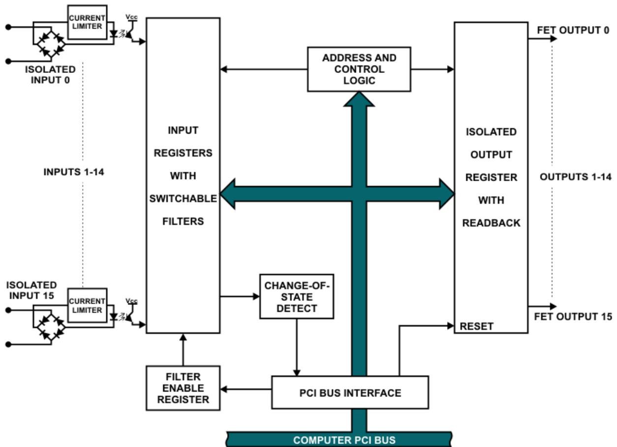
Figure 1-1: Block Diagram
