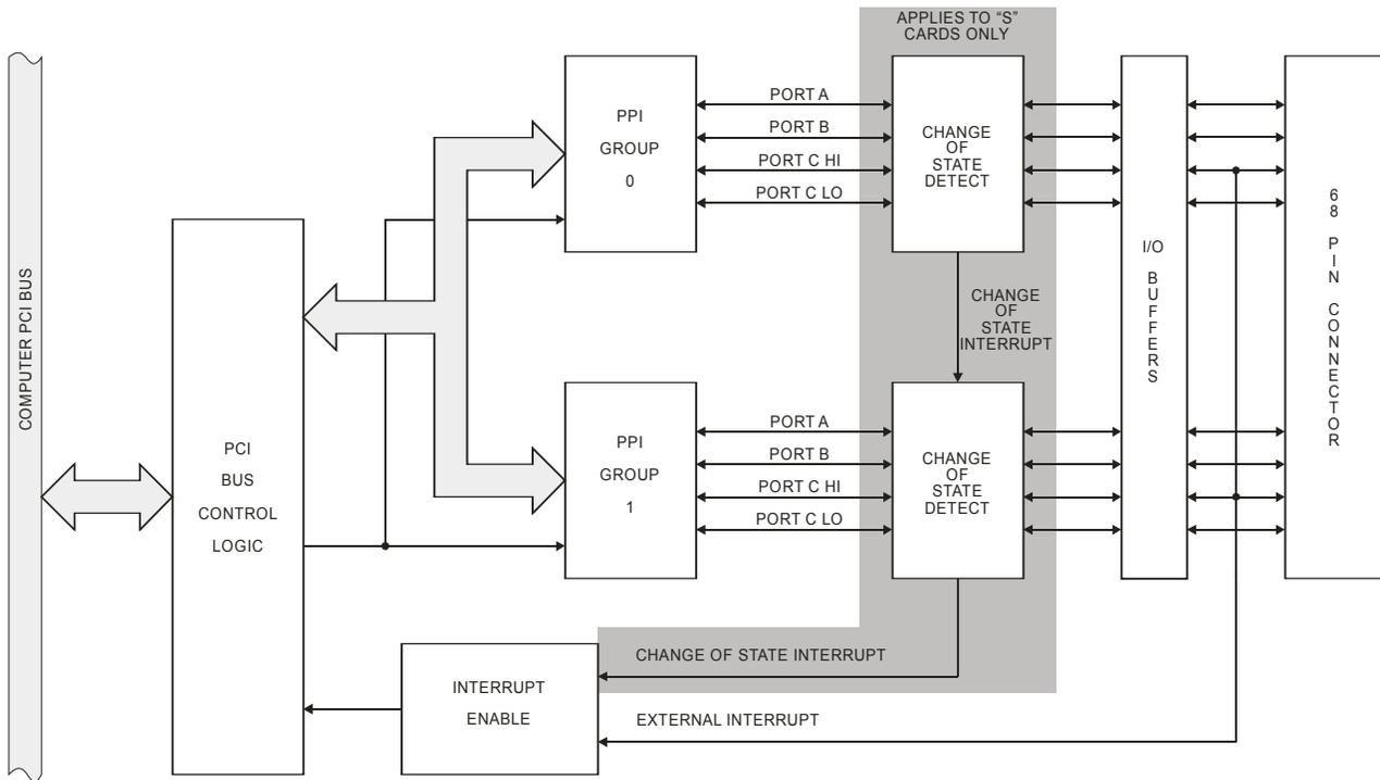
**Figure 1-1: Block Diagram**
