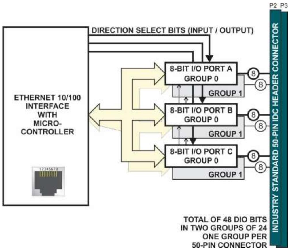
Figure 1-1: Block Diagram
